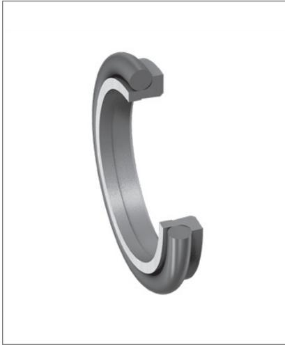
The function of wiper rings is to prevent dust, dirt, grains of sand and metal swarf from penetrating into axially moving rods and plungers. Thus the development of scratches is largely prevented, guiding elements and seals are protected and the working life of the sealing system is extended.
