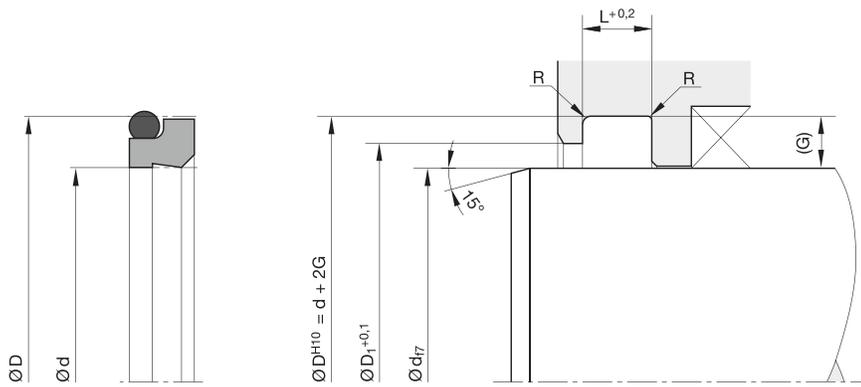
For surface finish, lead in chamfer and other installation dimensions see „General installation guidelines“.
