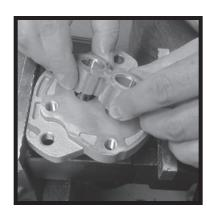
8) Carefully remove the bushing blocks from the bottom of body. Examine and replace if necessary. (See page 12)
