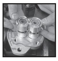
5) Mark bushing blocks top and bottom. Remove the bushing block. Examine and replace if necessary. See wear guide page 12.
