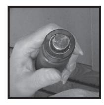
2) Place a new shaft seal on the installation tool with the spring side facing outward.
