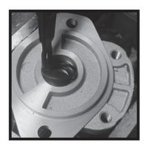
4) Assemble the snap ring. A new snap ring should be used if supplied in the seal kit.
