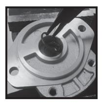
**9)** Remove the snap ring (located in front of the shaft seal).
