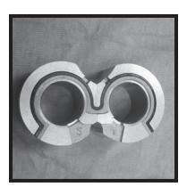
6) Assemble new sealing parts, the rubber seal first, the plastic seal on top. (Pump thrust block shown with seals installed.)
