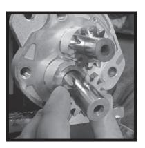
7) Carefully remove the drive and driven gears. Avoid tapping the gear teeth together or against other hardened surfaces. Examine and replace if necessary. (See page 12).
