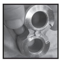
**11)** Inspect all bushings for scoring or discoloration and replace if necessary.
