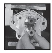
**11)** Install idler gear into thrust block and mounting flange.
