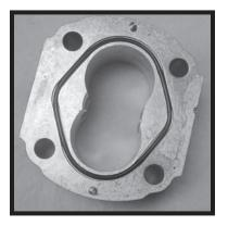
5) Check the section seal. Use of a new one is recommended in each case. Grease the new section seal to hold it in the groove.
