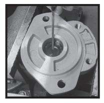
**10)** Pry out the shaft seal. Be careful not to damage seal bore in flange.
