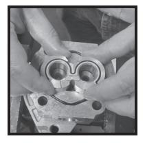
**14)** Install rear thrust block. Direction is important.
