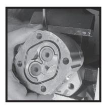
4) Remove gear housing. If prying is necessary, be careful not to damage the machined surfaces.
