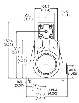
Note: 41.9mm (1.65") from bottom of bolt hole counterbore to bottom of valve.
