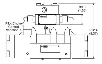
Note: 57mm (2.24") from bottom of bolt hole counterbore to bottom of valve.
