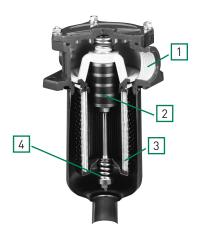
BGT Filters feature Parker's exclusive Magnetic Prefiltration core which collects ferromagnetic particles from fluid upstream of the filter element. This feature alone could save hundreds of dollars a year by protecting costly equipment from increased wear and malfunction by assuring that the fluid is as pure as possible when it leaves the filter. Even during bypass due to cold start up, ferris contaminant is collected by the magnetic core, a feature of importance on any fluid power system.
