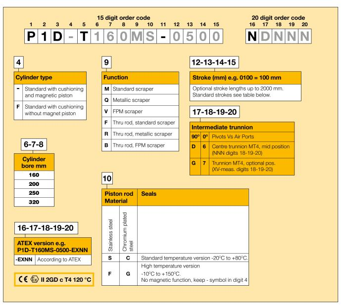
Order Key Code (Model code with 20 digits used only for the trunnion option or for the ATEX version)
