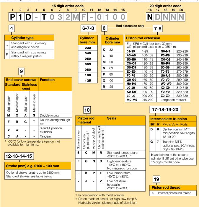
Order Key Code (Model code with 20 digits used only for the trunnion , female thread on the piston rod or to specify second cylinder stroke)
