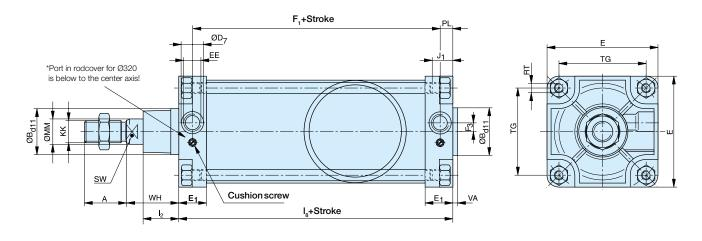
**Note \*:** for bore size 320mm, front air port is on the bottom of the axis of the cylinder and the cushioning screw on the top
