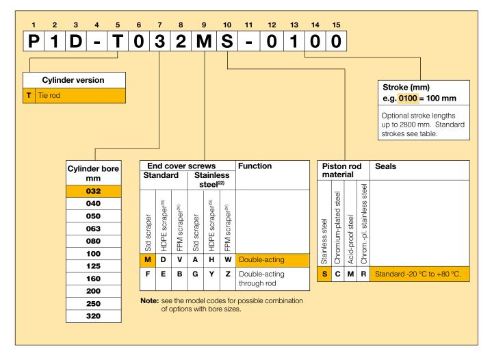
22) If stainless steel end cover screws are selected, the piston rod nuts are also supplied in stainless steel.
