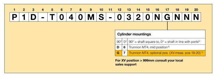
5) Shaft or pivots square to or in line with the cylinder ports.
