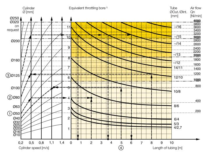
The "equivalent throttling bore" is a long throttle (for example a tube) or a series of throttles (for example, through a valve) converted to a short throttle which gives a corresponding flow rate. This should not be confused with the "orifice" which is sometimes specified for valves. The value for the orifice does not normally take account of the fact that the valve contains a number of throttles.
