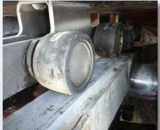
THIELE roller installed as an outside unit on a chain assembly.
