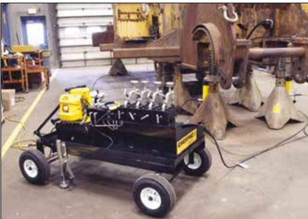
◀ Level Lift System provided a safe, fast lifting solution during the rebuild of an off-highway vehicle.
