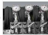
**Level lift valve.**4 outlets, lift and lower.
