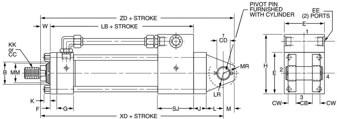
**Cap Spherical Bearing**
