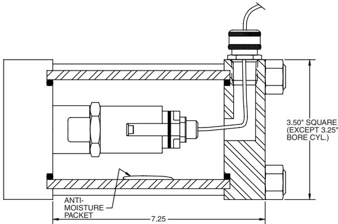
**Style D** — For LDT Basic and Integral Cap. Specify connector type (not available on 2" bore).
