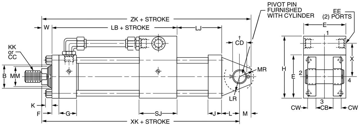
**Cap Spherical Bearing**
