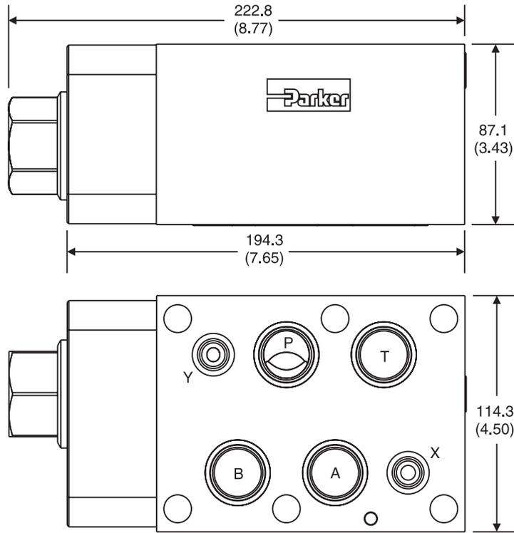
**CP08DD** – Inch equivalents for millimeter dimensions are shown in (\*\*)
