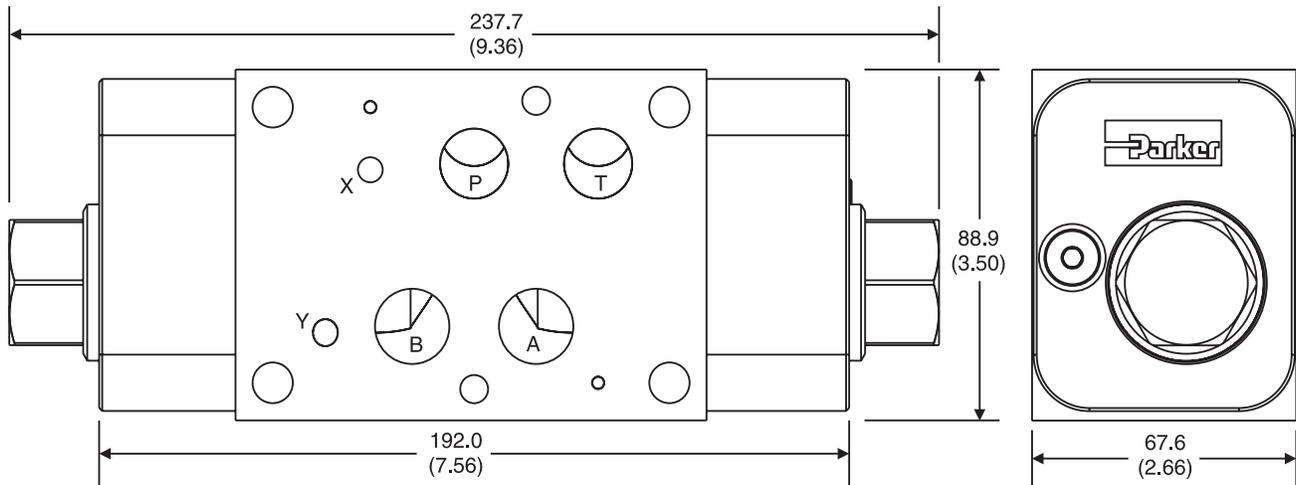
**CP08AA** – Inch equivalents for millimeter dimensions are shown in (\*\*)
