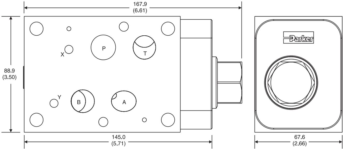
**CP07BB** – Inch equivalents for millimeter dimensions are shown in (\*\*)
