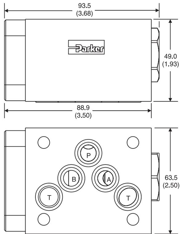
**CP05DD** – Inch equivalents for millimeter dimensions are shown in (\*\*)
